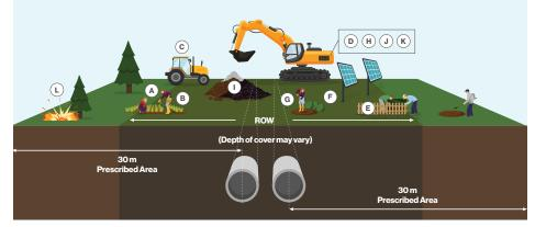
Enbridge Gas' cross-border and interprovincial pipelines are regulated by the Canada Energy Regulator (CER) and must comply with specific pipeline standards and regulations. In addition to the ROW where the pipeline is located, the CER has established a 30 metre prescribed area on either side of the pipeline to protect the public, the environment and the pipeline. More information about CER requirements can be found at cer-rec.gc.ca.
